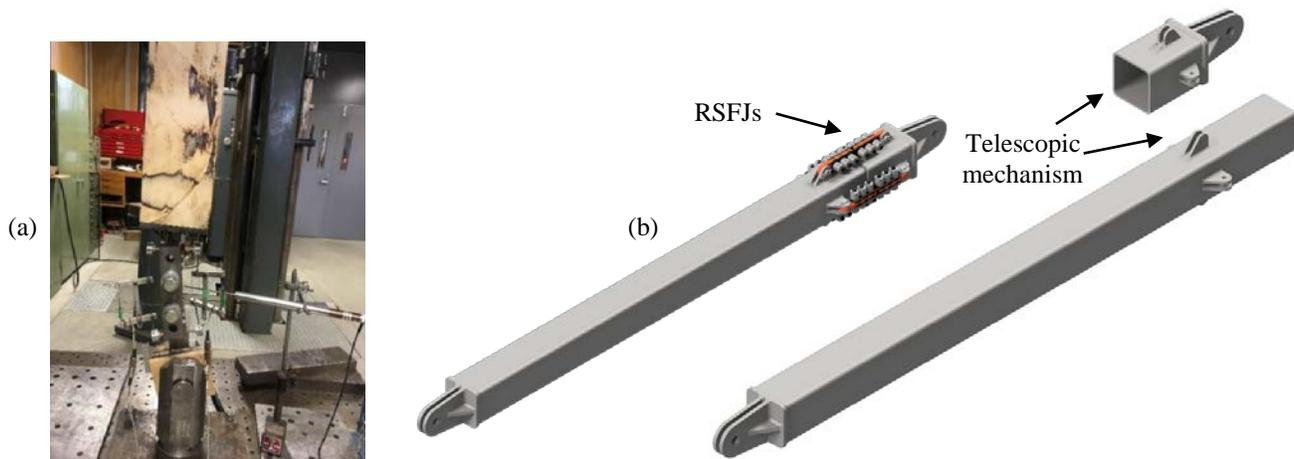
Figure 6. RSFJ brace: (a) experimental test, (b) telescopic mechanism
