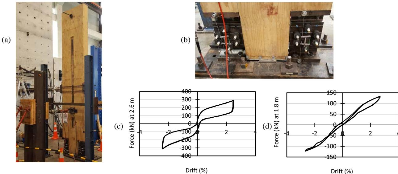
Figure 5. Full-scale testing of the rocking LVL column with RSFJ hold-downs: (a) test setup, (b) RSFJ hold-downs, (c) bi-directional test results, (d) out-of-plane test results
