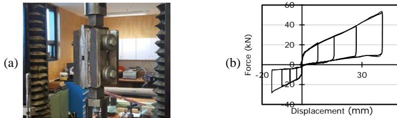
Figure 2. RSFJ component test: (a) test setup, (b) results of the cyclic tests
