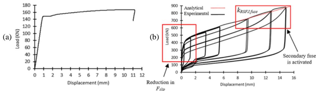
Figure 10. Experimental results of the RSFJ with the collapse prevention fuse: (a) load-deformation curve of the M18 rod grade 8.8, (b) load-deformation curves of the RSFJ
