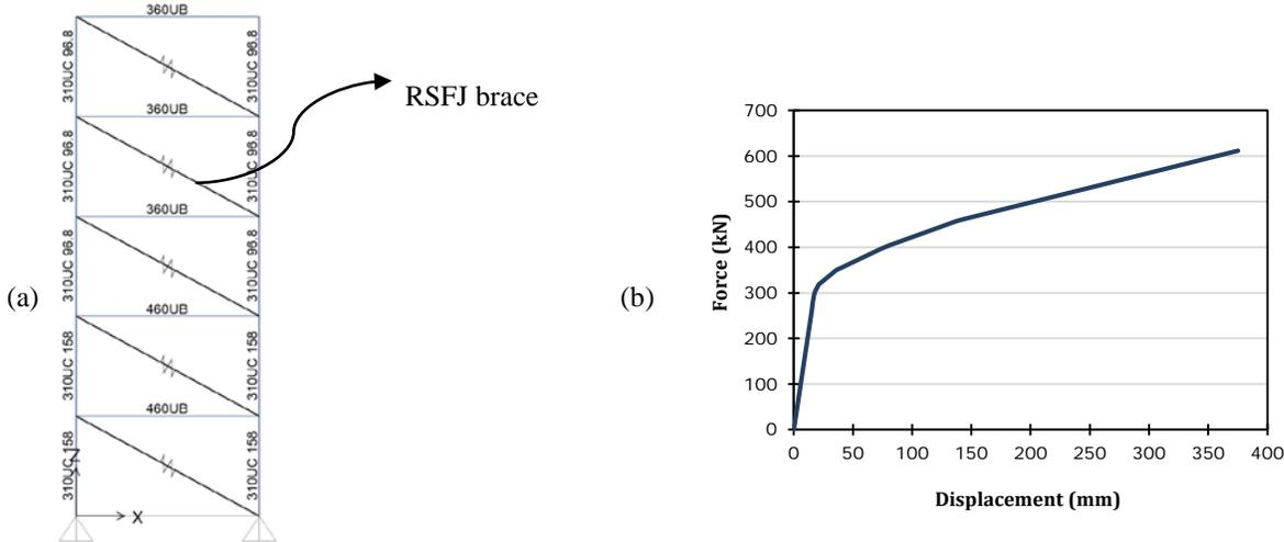
Figure 7. Numerical modelling of the prototype steel frame with RSFJ braces: (a) numerical assembly (b) push-over curve
