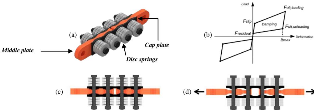
Figure 1. Resilient Slip Friction Joint (RSFJ): (a) assembly, (b) hysteresis, (c) the joint at rest, (d) the joint at the maximum deflection within its elastic response
