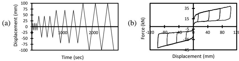
Figure 4. Test results: (a) applied load-schedule, (b) load-deformation behavior
