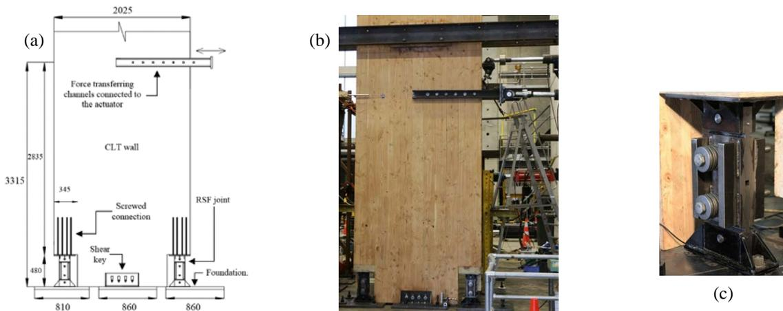
Figure 3. Experimental test of rocking CLT wall with RSF joints: (a) general arrangement, (b) test setup, (c) RSFJ
