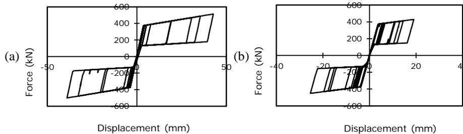
Figure 8. Numerical results: (a) RSFJ brace hysteresis for Kobe (MCE), (b) RSFJ brace hysteresis for Northridge (MCE)
